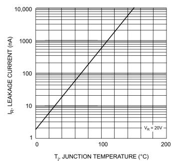
Fig. 2 Leakage Current vs Junction Temperature
