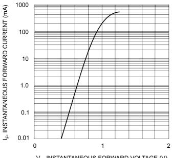
V<sub>F</sub>, INSTANTANEOUS FORWARD VOLTAGE (V) Fig. 1 Forward Characteristics
